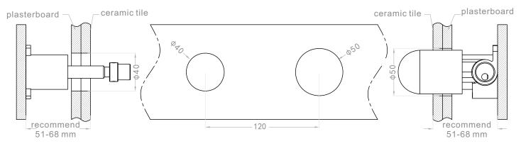
1. Fix body on noggin and ensure installation depth is 51-68mm from noggin to ceramic tile.
