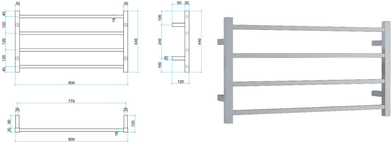
This rail has Multiflex wiring which means that there is a connection point on both the left and right hand side of the rail and the lead can be connected to either side. Being a dry electric element rail, this can be mounted either way up meaning the wiring can be from any of the four mounting points.
