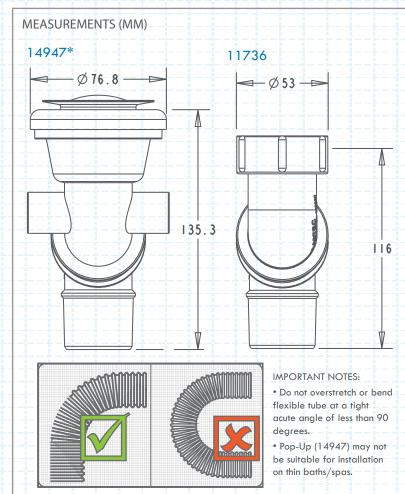
DO NOT OVERSTRETCH OR BEND FLEXIBLE TUBE AT A TIGHT ACUTE ANGLE OF LESS THAN 90 DEGREES.
