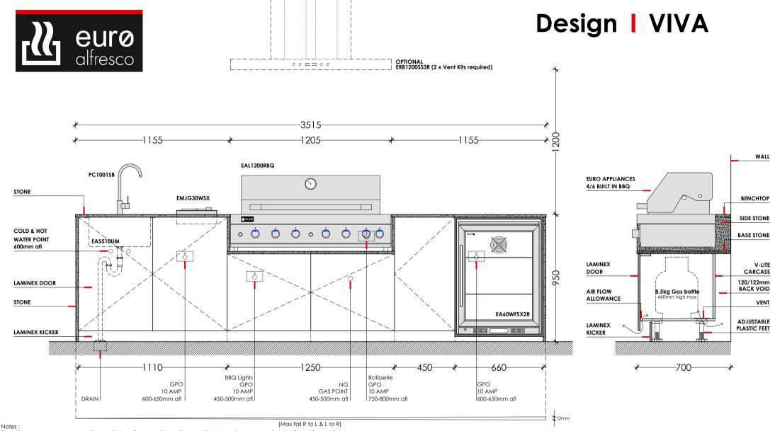
The alfresco area must comply with your States - Gas Acts, Regulations and Standards to be able to install a Euro Alfresco kitchen. Quoted for standard waterfall stone ends of 930mm high. It should be noted that a non-level surface will require a custom waterfall stone end to be cut, incurring an additional fee.
