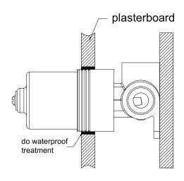
7.Do waterproof treatment for gap of plasterboard and body.
