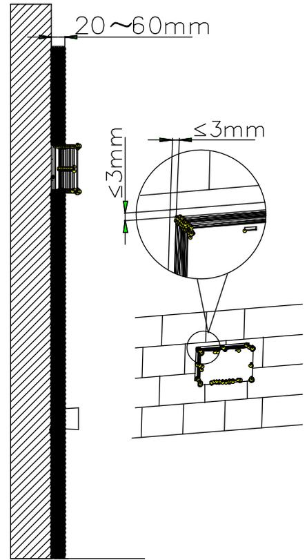
7. Installation of straight tube
