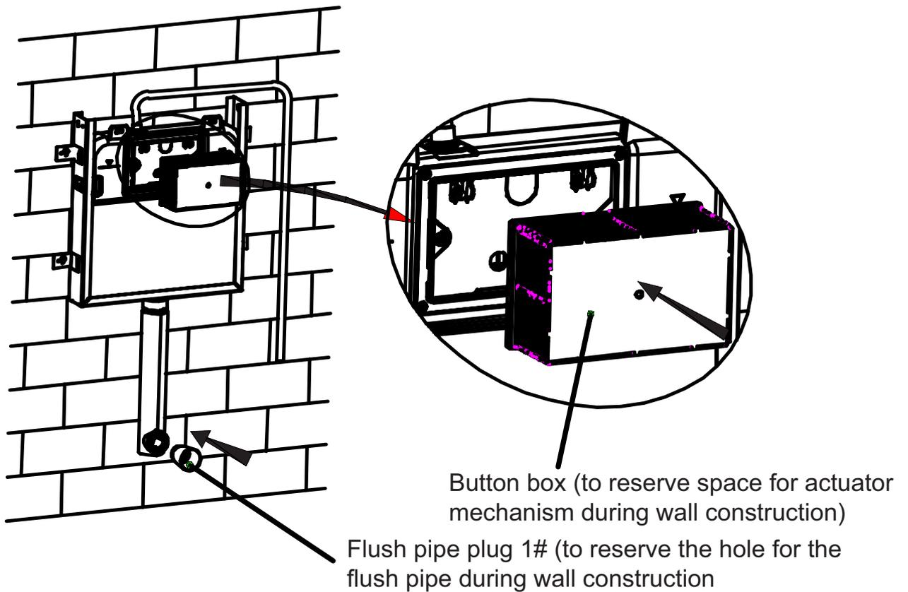
6. Wall thickness range 20-60mm (from frame outside surface to finished wall)
