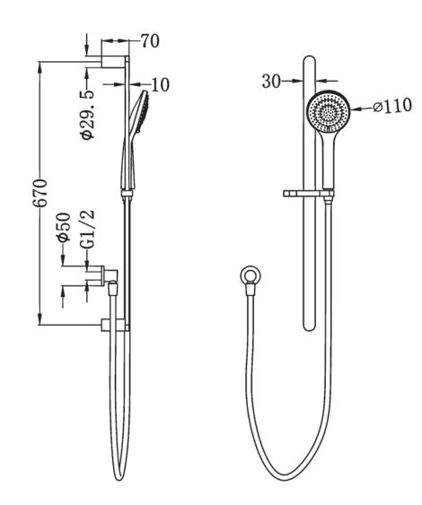
2. The inlet of the shower hose is connect to a wall elbow installed by the plumber at a suitable height. 4. This product may not be suitable for use with gravity-fed water heaters, low pressure supply networks, instantaneous water heaters, tempering valves and thermostatic mixing valves.
