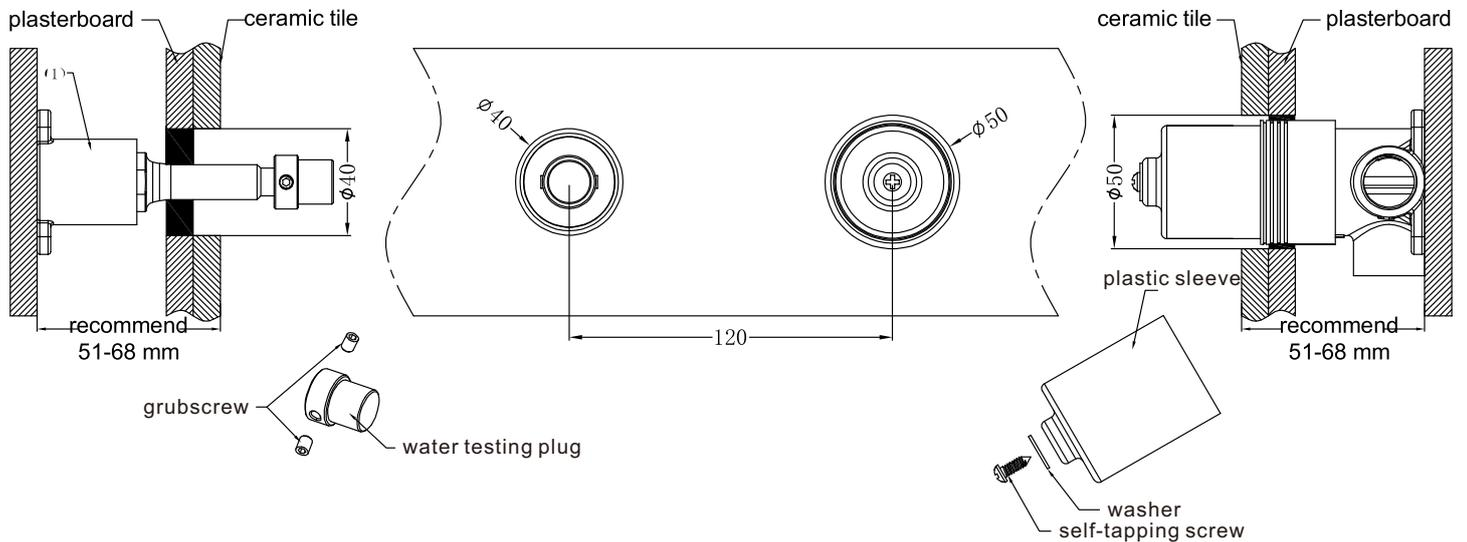
1. Drill a  $\phi 50$  and a  $\phi 40$  hole on ceramic tile, then install ceramic tile according to above picture.
