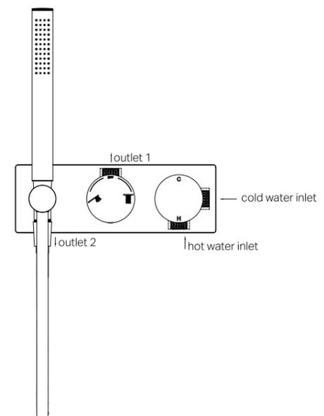
12. Installation is now complete. Test for leaks.
