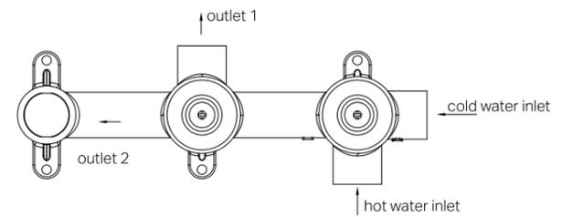
1. Fit off in-wall mixer body into wall structure, and ensure the installation depth is 51-66mm from the tile surface.
