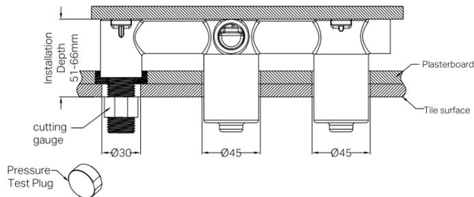
1. Install tiles and drill holes with diameters of Ø30, Ø45, Ø45.
