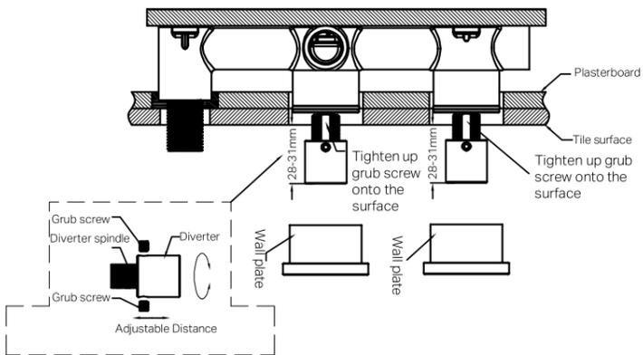
5. Adjust the distance between the Diverter knob and the tile surface to 28-31mm, as shown in the diagram.
