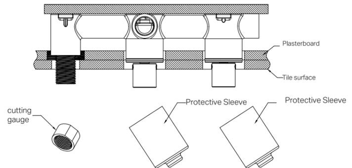
4. Remove the cutting gauge and protective sleeve.
