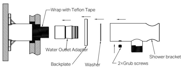
8. Thread the water outlet adapter onto the in-wall body, and seal with Teflon tape.
