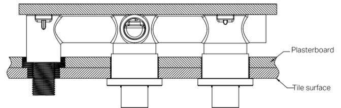
7. Apply waterproofing in the gap between the ceramic tile and the water outlet.
