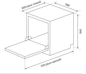
\* Height can be reduced to 815mm for built-in installation. See the user manual for detailed ventilation and installation details.
