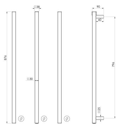
Electricity Input: 12V | Power Rating: 35W | IP Rating: IPX5 | Connection position: Bottom right | Connection type: Hardwire
