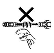
Never twist or stretch the flexible hose during installation.
